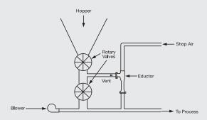
In existing installations that employ rotary valves, solids handling eductors have been proven to improve performance and efficiency. They deliver considerable economic benefit by venting and recovering blowback air and product using existing shop air at 50-80 psi. Solids handling eductors can recycle solids back to the feed bin or boost vent air directly into the conveyor line. They are commonly employed in both single or double airlock installations to extend air lock life.
