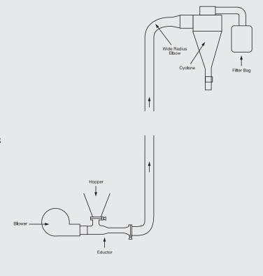
The absence of moving parts creates the opportunity to convey sensitive materials with less damage. Plastic pellets suffer less chipping, activated carbon experiences less degradation, and pet foods are transported with less product loss. Additionally, solids handling eductors can be employed in sanitary installations for a fraction of the cost of rotary valve technology.
