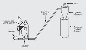
Solids handling eductors are ideal for conveying product from bag dump stations. Food additives (sanitary dump stations) and fine powders (talc, resins) are examples of bag dump applications that benefit from eductor technology. Placed below the hopper in a bag dump station, eductors eliminate blowback due to leakage and control dust clouds by creating a vacuum and drawing the product in. The result is an improved work environment.
