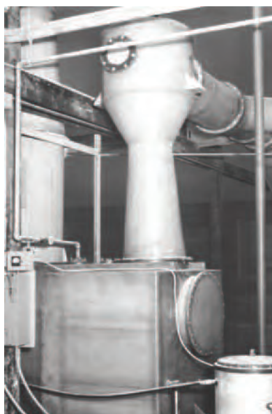
Fig. 7014 scrubber-separator system removes sulphur monochloride. It is part of a multi-unit system using a mild caustic as the scrubbing liquid.
